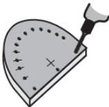
Using a PROTRACTOR, measure off the center point, and mark points at 15 degree increments along the inner line (FIG 16).
