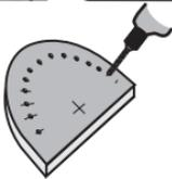
Using a KEYHOLE SAW, cut along the outer edge.
